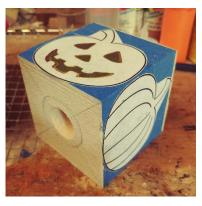
**STEP 1:** The blank I am using is 3"x3"x3" Basswood. Start the Pumpkin project by preparing the blank. Measure the height of the Tea Light and drill a 1-inch hole in the center of the bottom of the blank. Recommend that the hole be at least ½ inch smaller than the diameter of the Tea Light base. This will be enlarged later to fit the base of the light.
