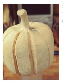
**STEP 7:** Using a knife of your choice, widen the groove slightly. The Stop Cut makes removing the waste wood easier. Sand the groove to round the edges of each segment.
