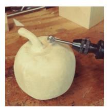
**STEP 4:** Carefully carve the stem to a more natural look. Slightly indent the area around the base of the stem using a ball cutter.
