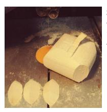
**STEP 3:** Round the blank using a method you are comfortable with. This can be carved or sanded. I cut off the corners to aid in the rounding. While rounding the blank, decide the shape of the pumpkin you desire to make.
